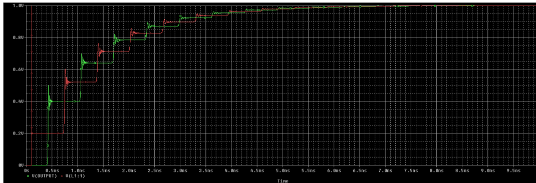
Figure 13: Simulation waveform of an open-circuited transmission line
