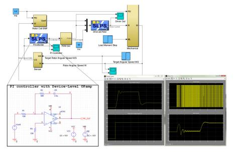
Figure 2: The PSpice SLPS interface enables you to interface the PSpice circuit with Simulink and then observe the waveforms after Simulink-PSpice co-simulation.
